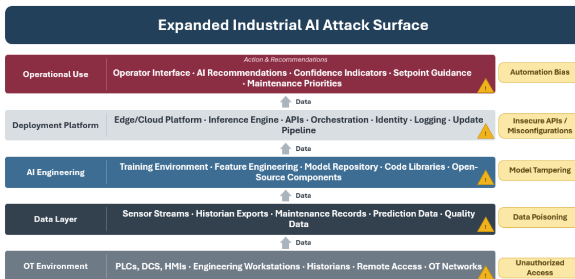
Figure 2 industrial AI attack surface examples and operator decision pathways.
